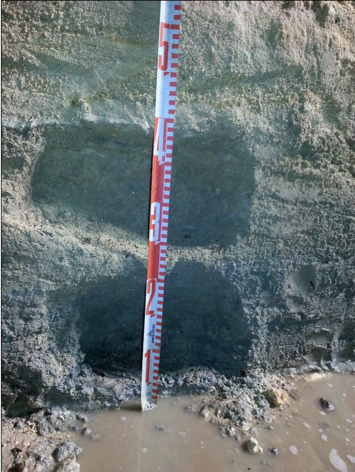
Figure 103. Close-up of the berm feature (SIHP # -7655) (Stratum II) overlying the wetland sediments (Stratum III) within the TE 16 southeast sidewall, view to southeast
