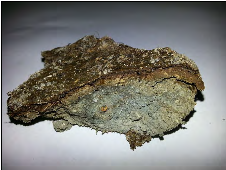
Figure 242. Close-up of TE 1 laminated organic material (Stratum IIb SIHP # -7655), showing distinct layering with leaf and organic material visible at the upper boundary
