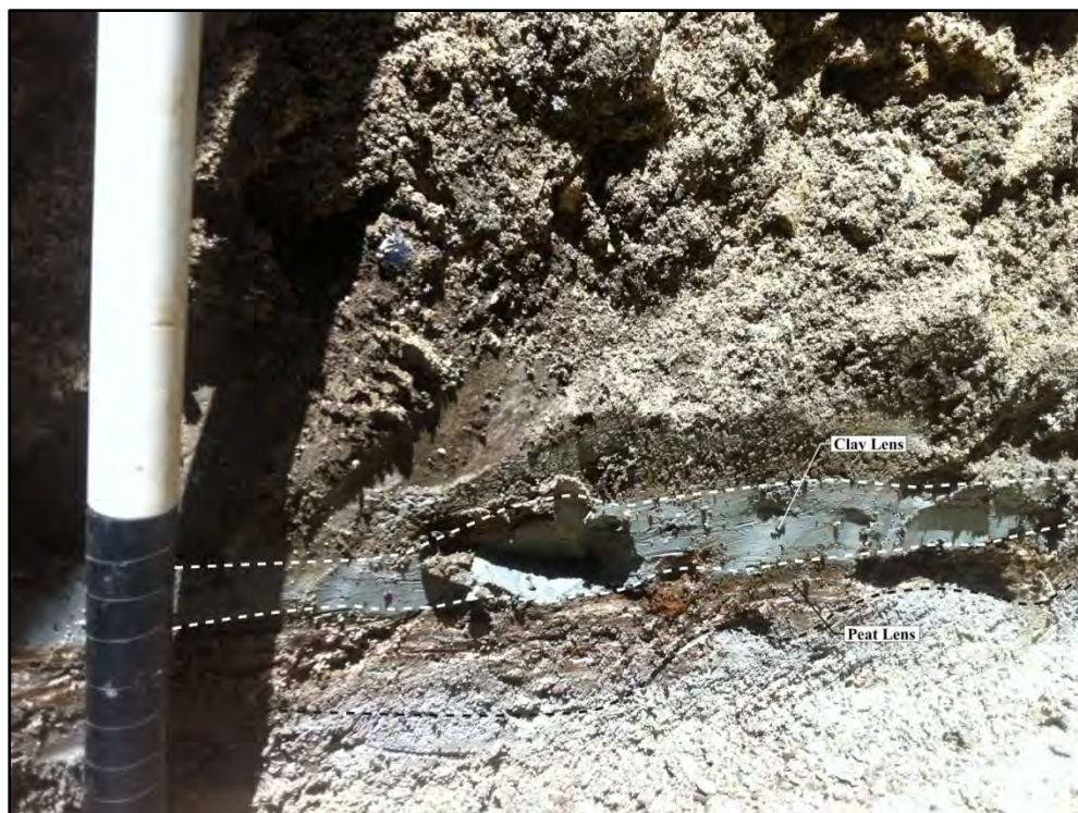
Figure 254. Photograph of T-230 (Hammatt 2013), showing Stratum II clay and peat salt pan sediments (SIHP #-7190)
