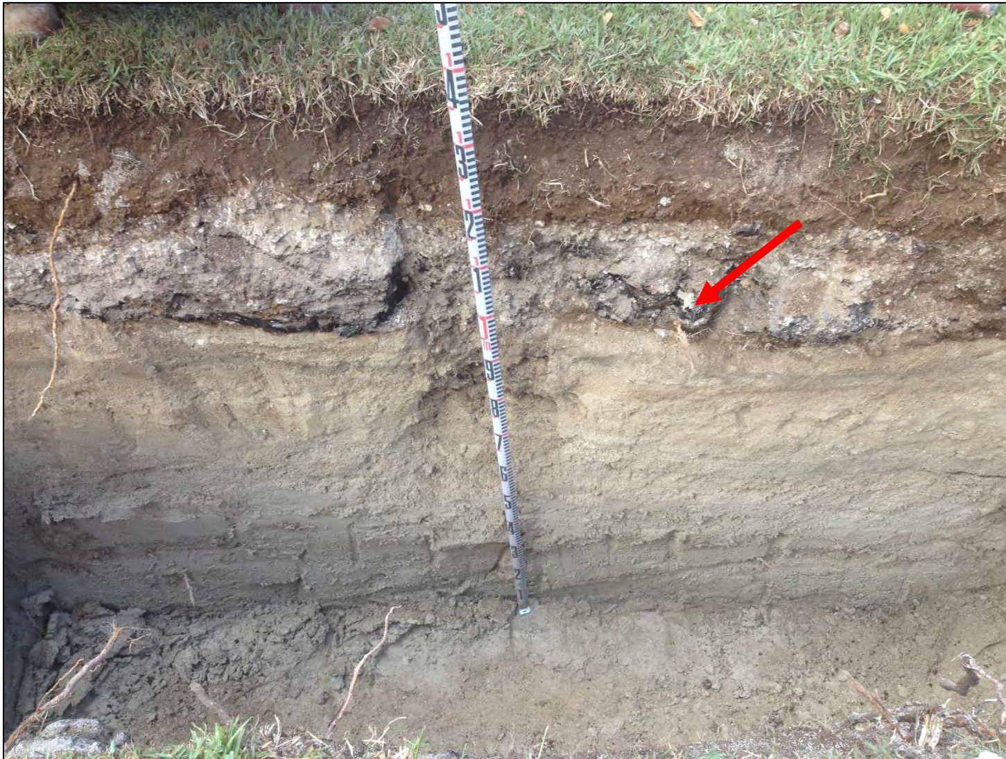
Figure 282. Photograph of a coral and tar buried surface (SIHP # -7658) within Block B East TE 30, indicated by the red arrow
