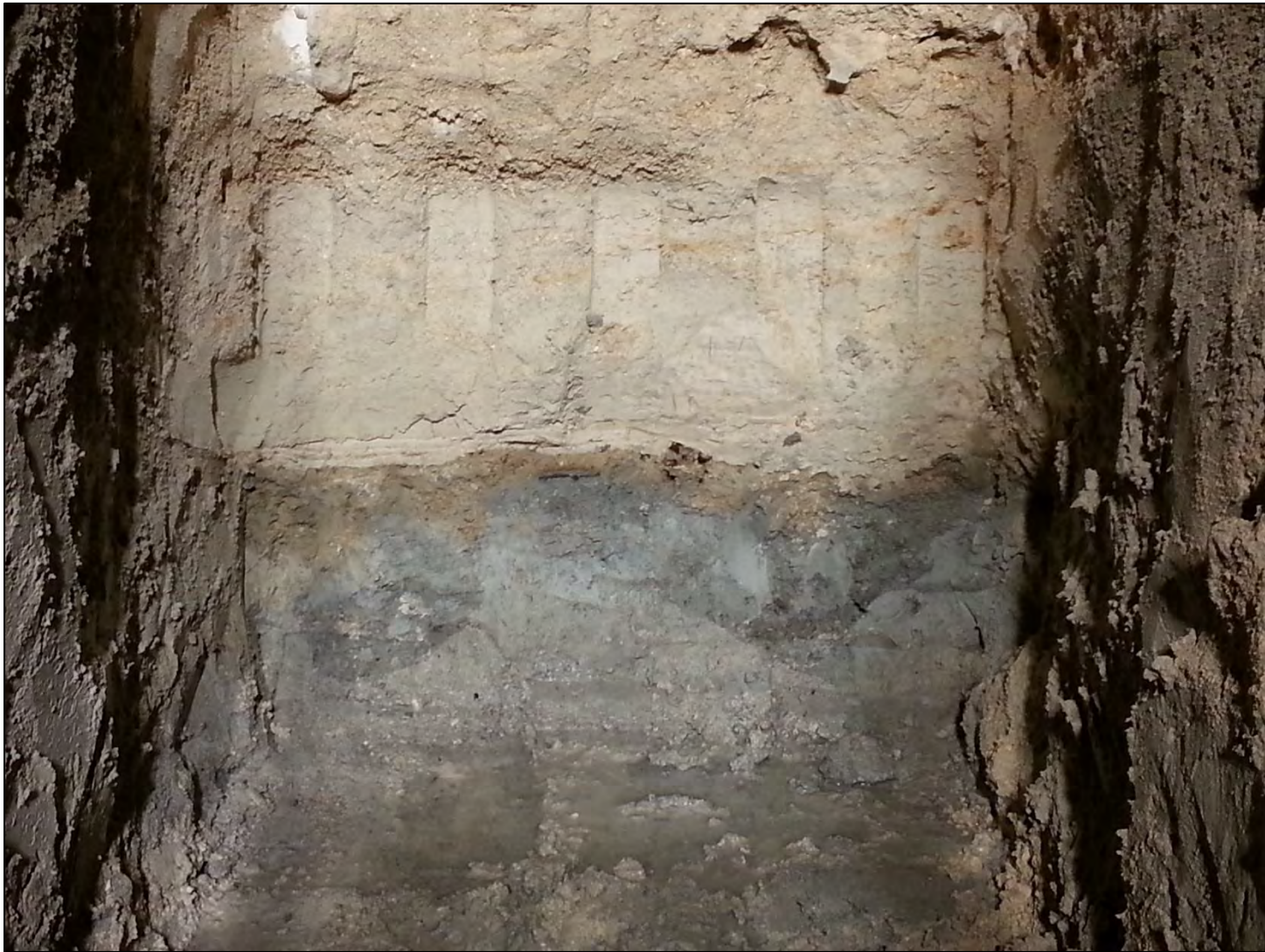
Figure 182. Close-up of northwest end of TE 37, showing the beginning of a transition from the man-made berm to a salt pan bed
