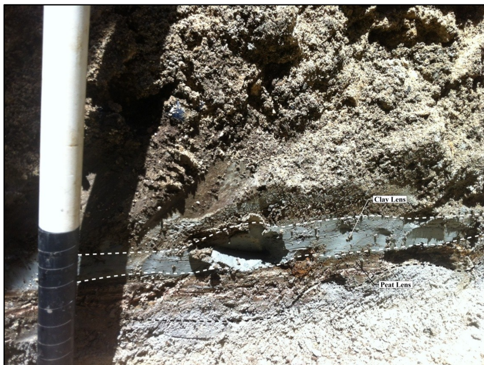
Figure 47. Photograph of T-230 (Hammatt 2013), showing Stratum II clay and peat salt pan sediments (SIHP #-7190)
