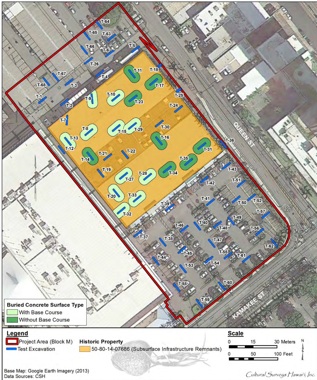
Figure 353. Aerial photo showing the locations of buried concrete surfaces with associated base course layers and concrete surfaces without associated base course layers (SIHP # - 7686) in the Block M project area
