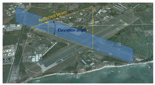
Fig 15.- Reflected beam elevation angle for Runway 29
