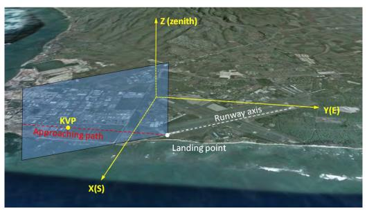
Fig 10.- Geometry of approaching path
