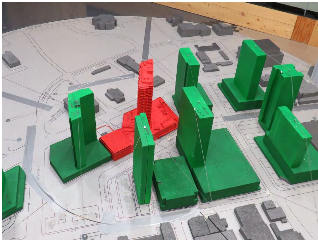
Wind Tunnel Study Model Configuration 2
