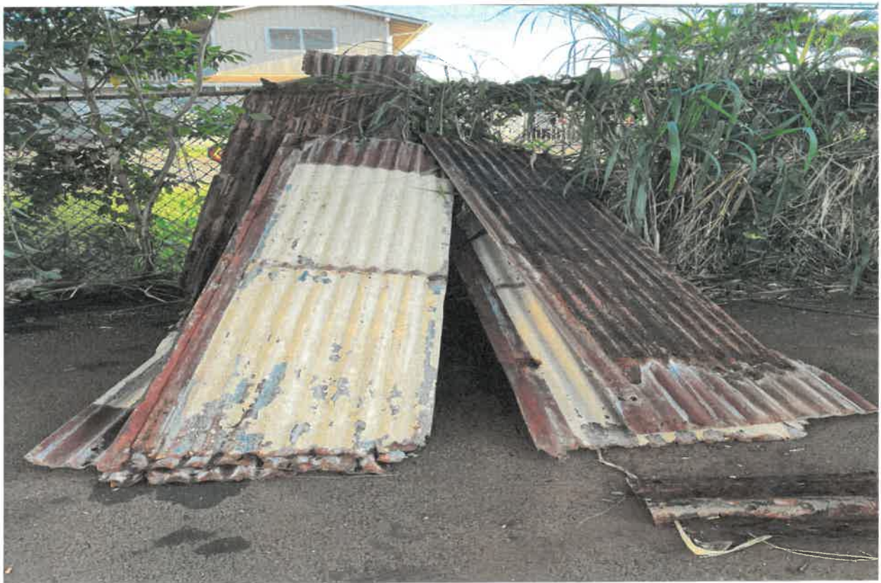
CORRUGATED METAL ROOF PANELS W/MULTI-LAYER ASBESTOS COATINGS.
