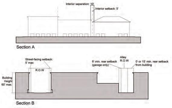
Figure D-31 Mixed Use Area Buildings with Storefront Section diagrams
