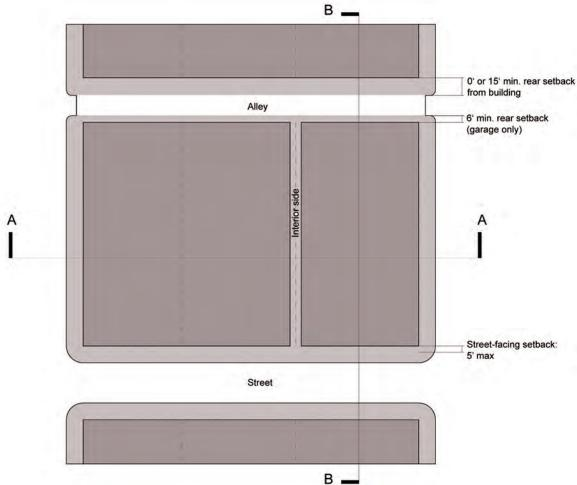
Figure D-30 Mixed Use Area Buildings with Storefront Plan diagram
