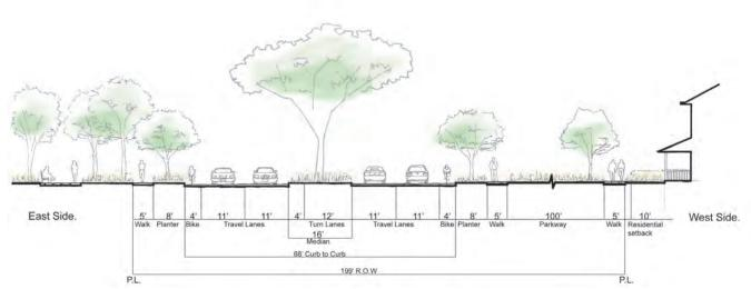
Figure D-12 Keoneula Connector Road Street Section
