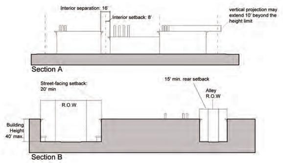
Figure D-44. Industrial Area Buildings Section Diagram
