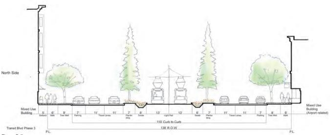
Figure D-7 Saratoga Road Street Section Phase 3
