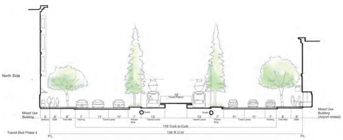
Figure D-8 Saratoga Road Street Section Phase 4
