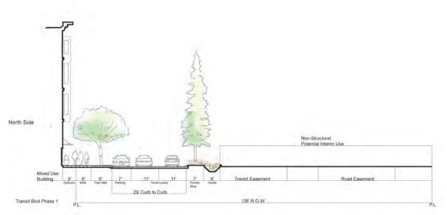
Figure D-5.Saratoga Road Street Section Phase 1
