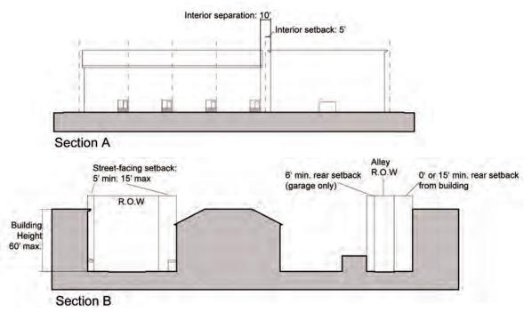
Figure D-34. Mixed Use Area Buildings without Storefront Section Diagram
