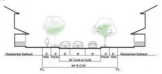
Figure D-23 Lane with Parking on 1 Side
