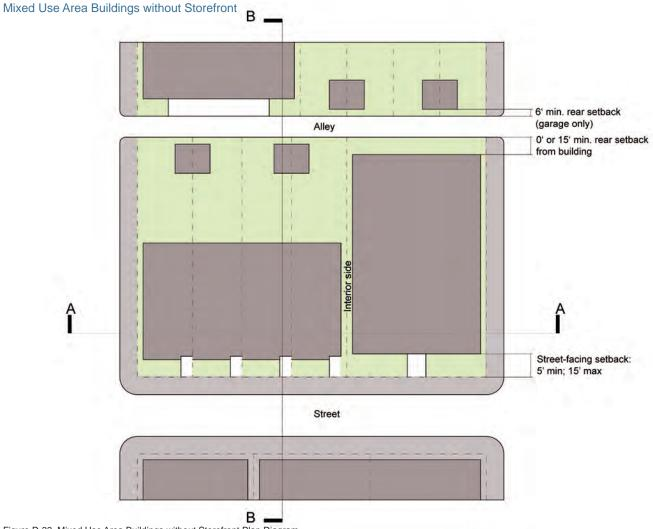
Figure D-33. Mixed Use Area Buildings without Storefront Plan Diagram
