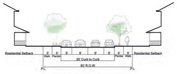
Figure D-22 Lane with Parking on 2 Sides
