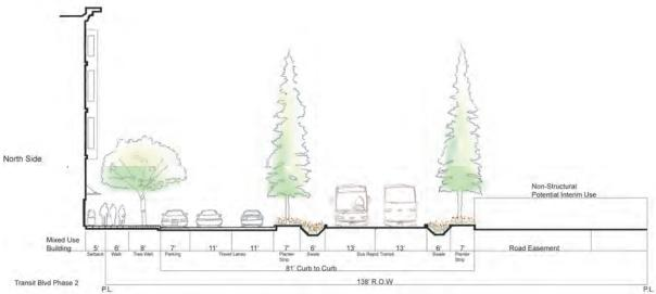
Figure D-6 Saratoga Road Street Section Phase 2
