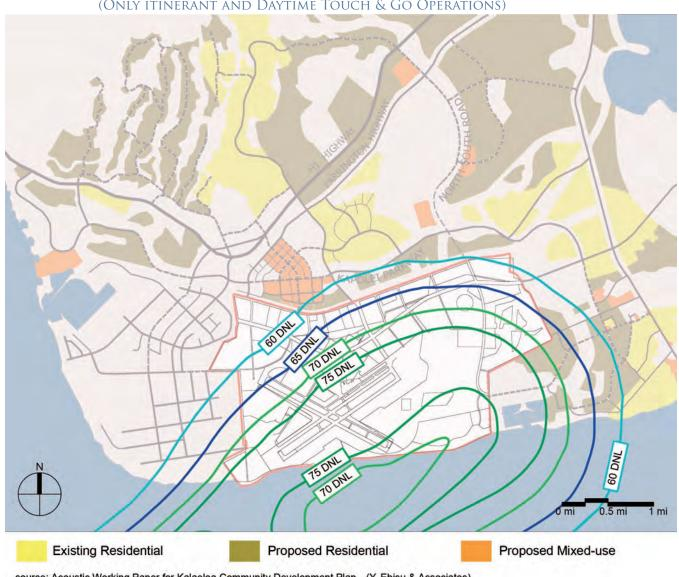
FIGURE F-4 FICTITIOUS JET FIGHTER AIRCRAFT NOISE CONTOURS AT KALAELOA AIRPORT (ONLY ITINERANT AND DAYTIME TOUCH & GO OPERATIONS)
