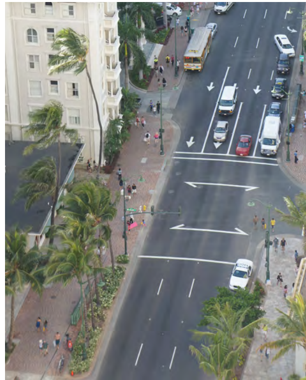
On Kalakaua Avenue in Waikiki, limited curb cuts and wide sidewalks help create a world-class pedestrian environment. Image from Nelson\Nygaard
