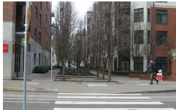
Both pedestrian streets shown above also provide mid-block access to parking facilities and are carefully designed to minimize the effect of auto access. This treatment eliminated curb cuts on the main street and allows enhanced pedestrian connectivity on these longer development blocks. Images from Nelson\Nygaard
