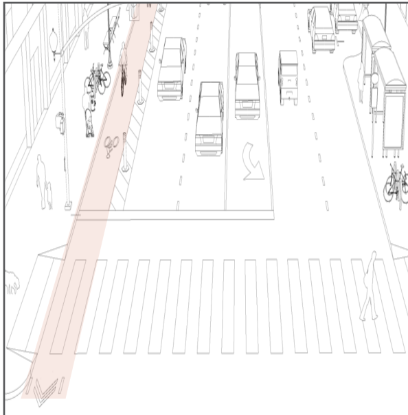
For South/Punchbowl Streets, one-way or two-way cycle track design could be implemented. Image from Nelson\Nygaard
