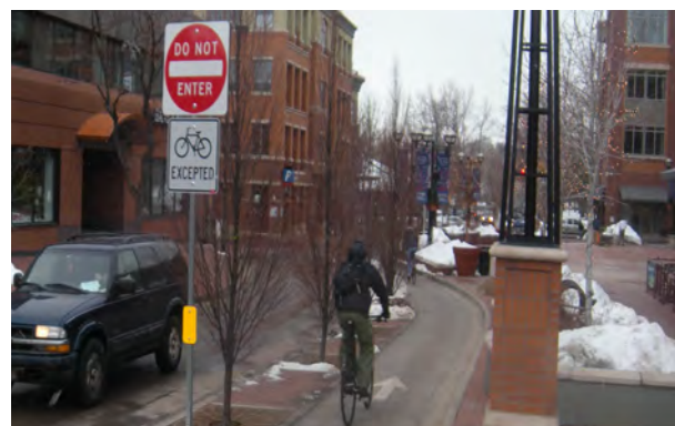
A pedestrian street in Boulder carries one-way traffic, includes a cycle track, and broad sidewalks. Brick treatment enhances the pedestrian zone. Images from Nelson\Nygaard
