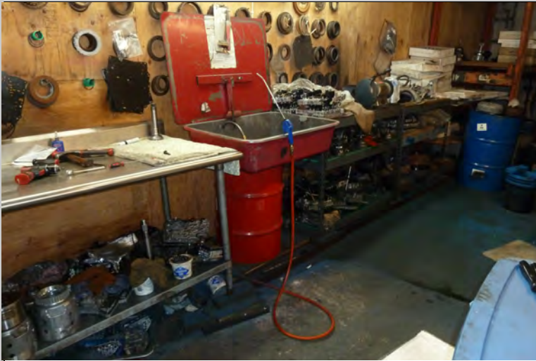
Photo 6: Wastewater from cleaning parts is collected in a 55 gallon drum in L & L Transmission.
