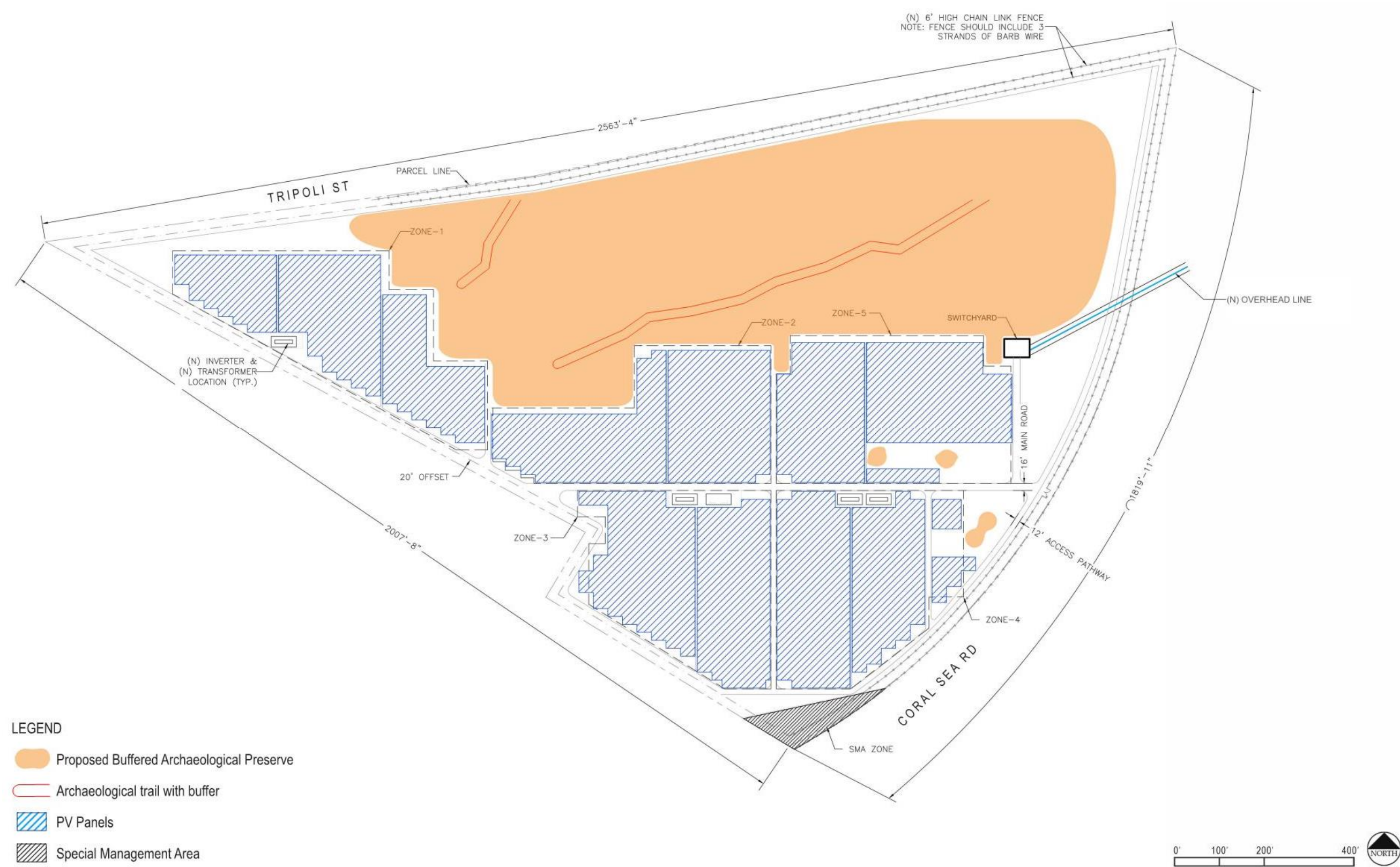
FIGURE 2-1 CONCEPTUAL SITE PLAN LAYOUT FOR PROPOSED 5MW PHOTOVOLTAIC UTILITY INSTALLATION WITH ARCHAEOLOGICAL PRESERVE
