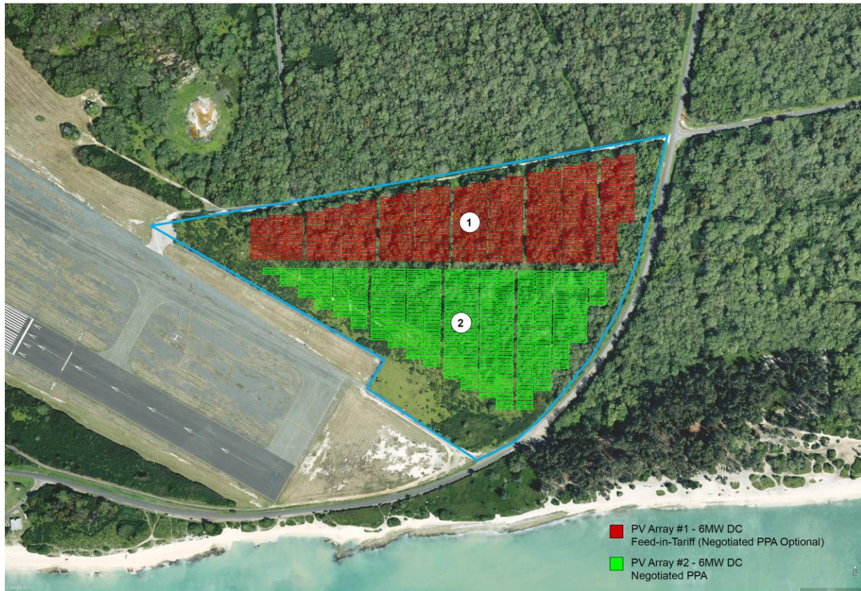
FIGURE 4-1 ALTERNATIVE SCALE OF INTENSIFIED USE – CONCEPTUAL 12.1 MW PV SYSTEM
