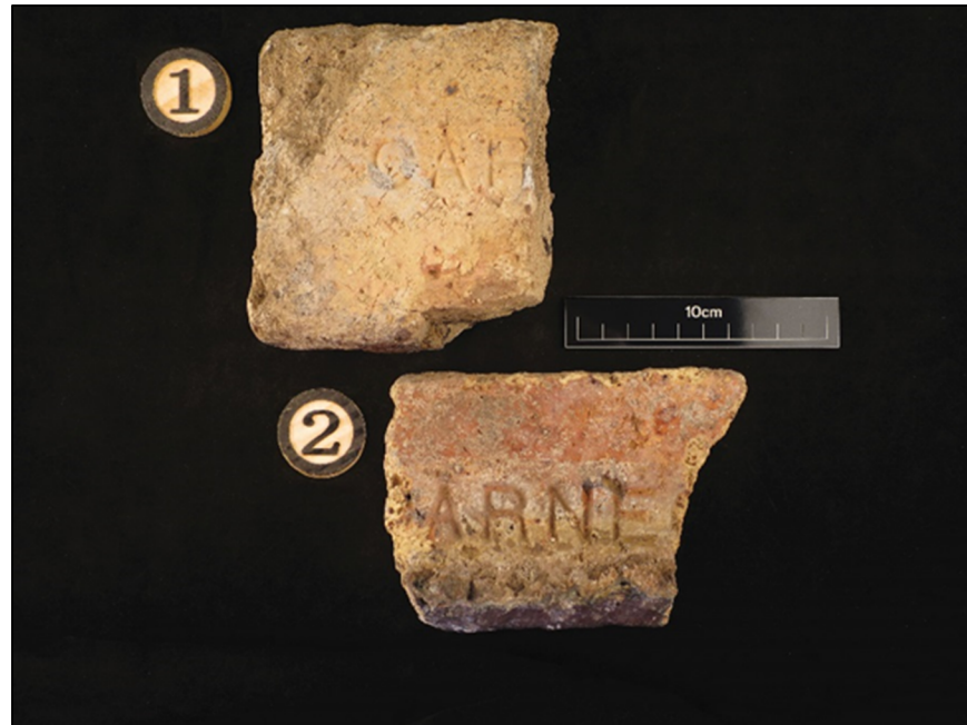
Figure 73. 1) Acc. # 37 and 2) Acc. # 38, Carnegie brick fragment, clay bar made with extruded, stiff-mud process and sent through Raymond and Berg cutting machine, brick made with patent pressed brick machine, impressed mark "CARNEGIE" on face, no frog, United States, 1903-1932
