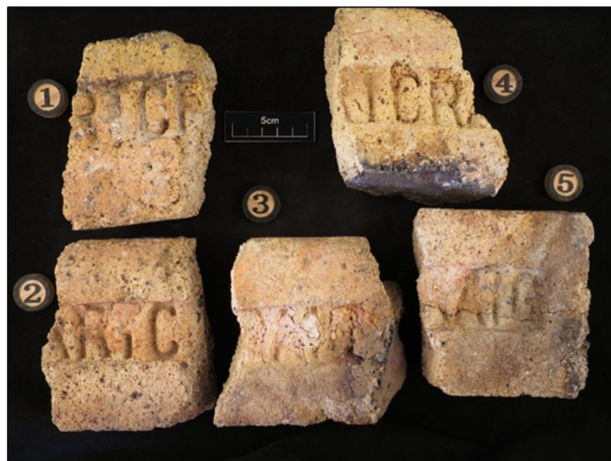
Figure 74. 1) Acc. # 39, 2) Acc. # 40, 3) Acc. # 41, 4) Acc. # 42, and 5) Acc. # 43, Gartcraig firebrick fragment, machine-made, impressed "GARTCRAIG" inside rectangular frog on face, Scotland, 1872-1921
