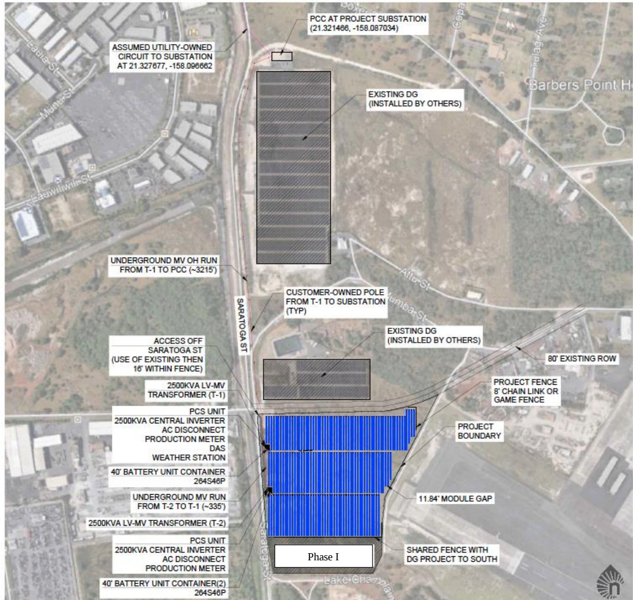
Figure 2: Conceptual layout for Photovoltaic system on the parcel at full capacity. Full capacity may not be obtained for 3-5 years and is dependent on the subscription rate and authorization from Hawaiian Electric.
