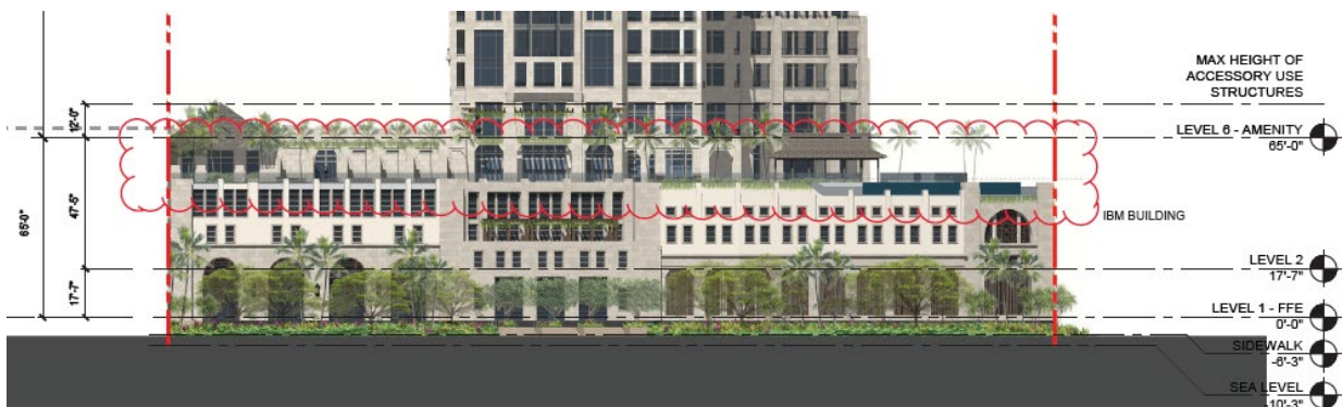
Image 3 – South elevation, parking podium height encroachment (Permit Application Exhibit 26)
