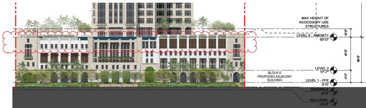
Image 3 – South elevation, parking podium height encroachment (Permit Application Exhibit 27)
