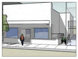
Figures 7.2 and 7.3: External wheelchair ramps accessed directly from sidewalk to ensure easy access. Ramps are located on the side of building (illustrative images).
