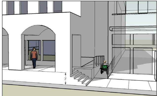
Figures 1.16-D and 1.16-E External wheelchair ramps accommodated under an arcade (illustrative images).
