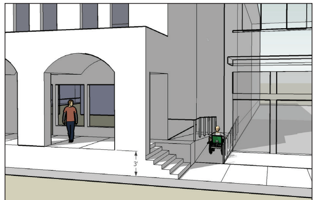
Figures 15-D (left) and 15-E (right): Illustrative external wheelchair ramps accommodated under an arcade
