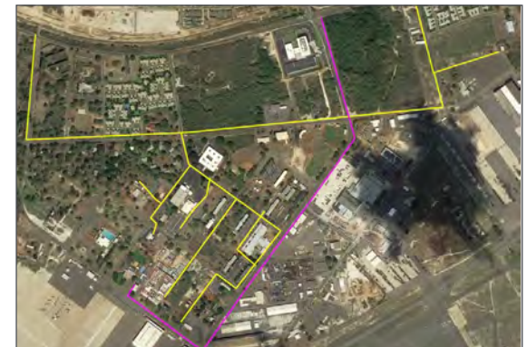
Figure 1-13: Electric Distribution Systems. Source: Electrical Distribution System Review (Draft Final), C.H. Guernsey Col., April 2020
