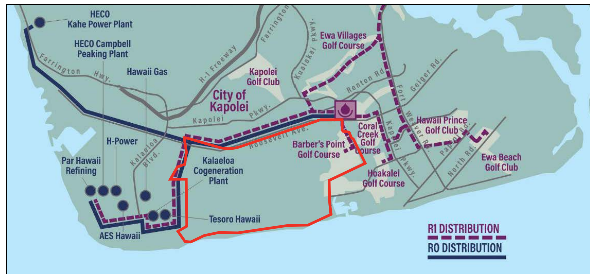
Figure 1-10: Ewa-Kapolei Recycled Water Distribution. Source: Board of Water Supply, City and County of Honolulu, March 2021
