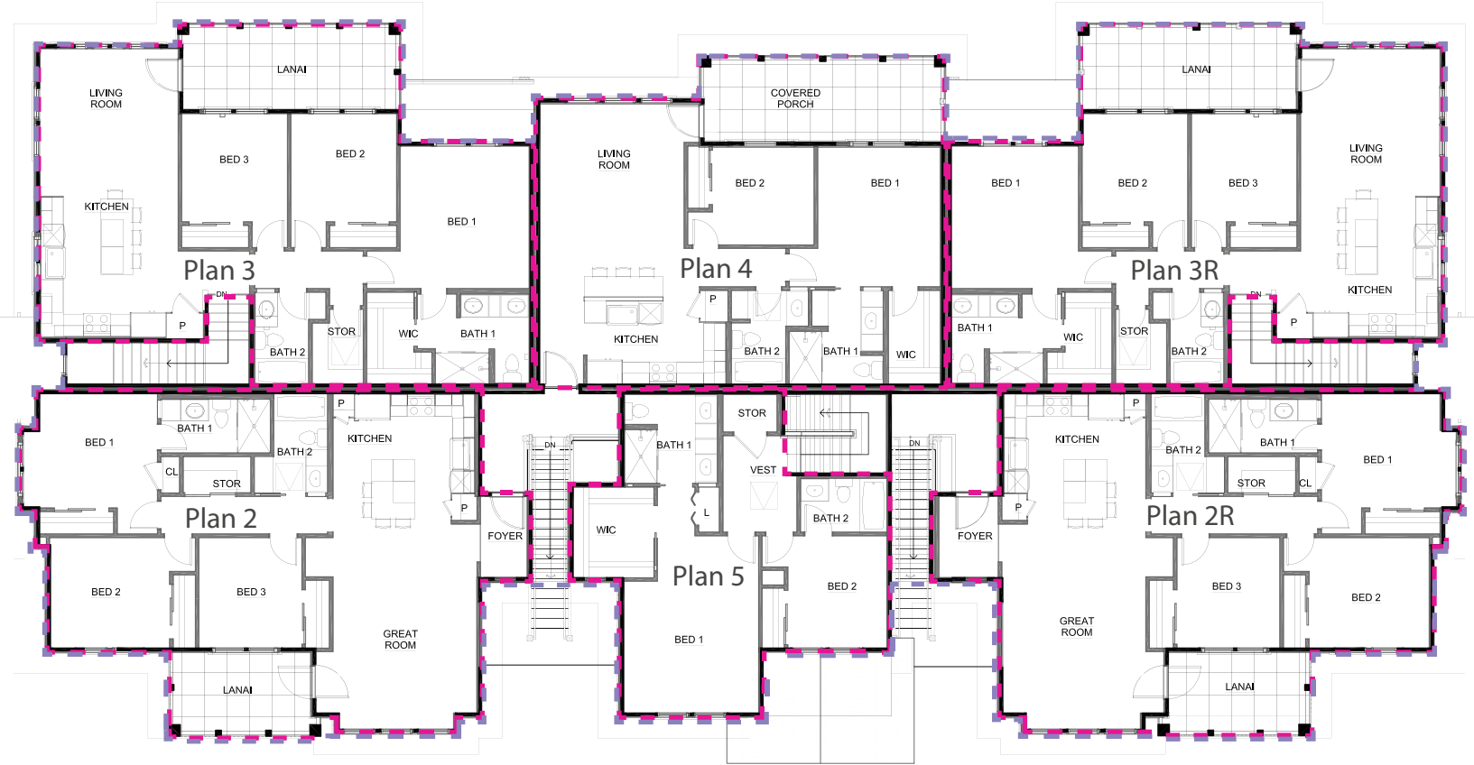
Second Floor Plan Flex Loft 8-Plex
