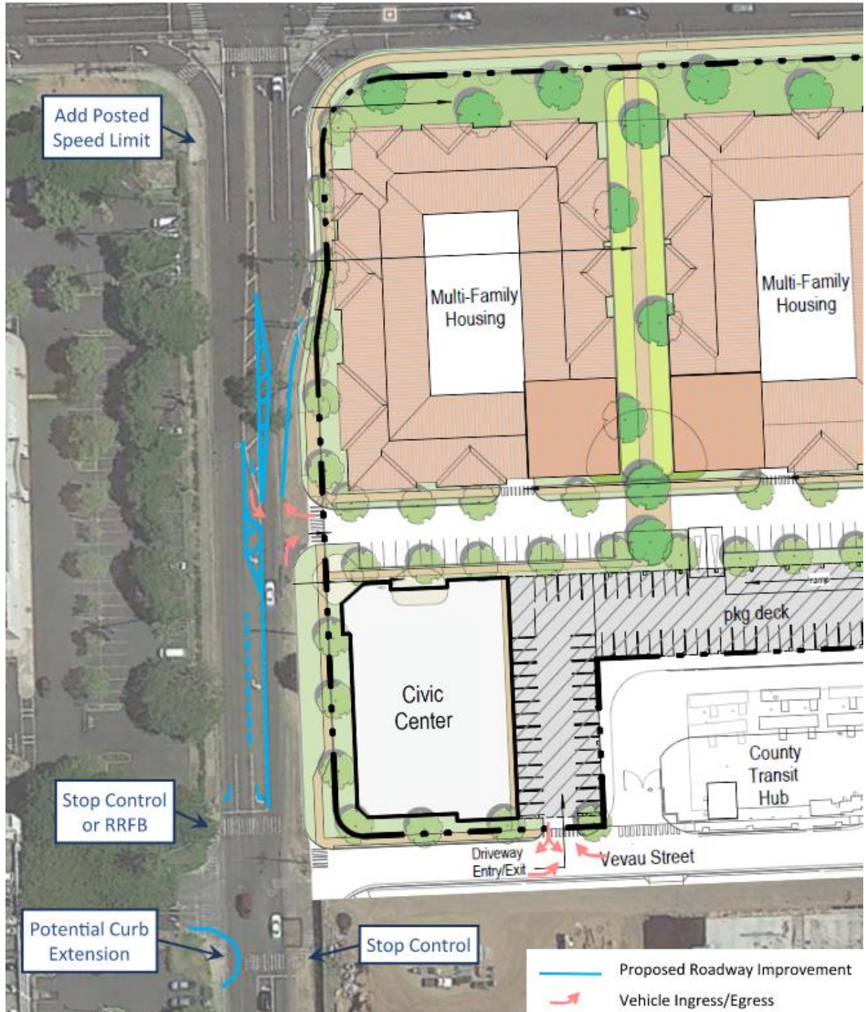
FIGURE 4: STRIPING AND ROADWAY IMPROVEMENTS
